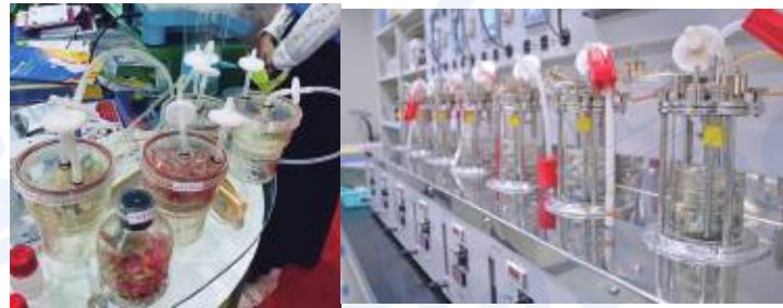
▲ Bio-reactor/ Fermentation air filters
